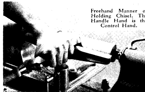
When the Chisel Is Held in This Manner, the Chisel Hand Controls the Cut.
