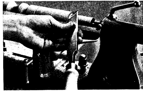
The Heel of the Skew Chisel Is Used in Making the Horizontal Cut Where It Joins With the Side Cut.
