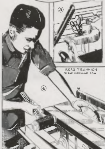
5. Check squareness of blade and make any necessary adjustment at stop screw. Repeat operation at 45° position. Check depth gage and angle gage, adjusting pointers to show proper reading.
