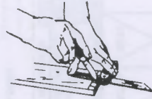
Duplicating lines drawn at the same angle, as in laying off dovetails for a drawer.
