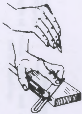
Laying off a mitre with a bevel.
